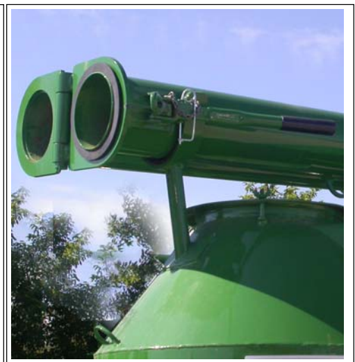
Fig. 14b BOOM FULLY COLLAPSED
